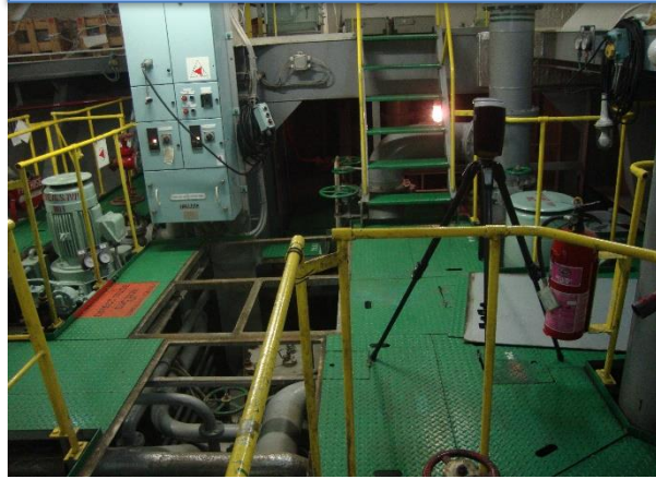
3D Scanning of Seachest Area – EGS-BWTS
